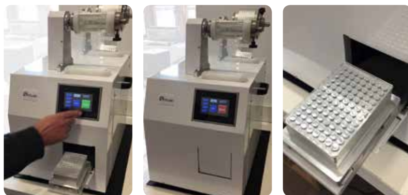
Figure 3: Random Access Sealing Procedure using the a4S RA Automatic Random Access Heat Sealer (4ti-0675, prototype shown)
